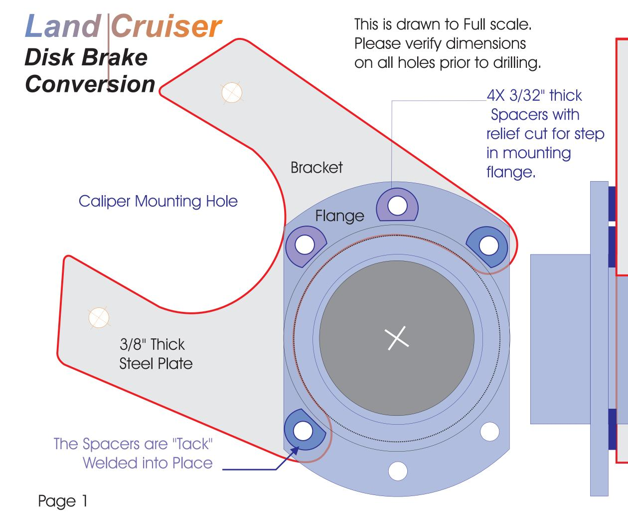
This is the Rear Disk Brake Conversion Bracket used with 1978 MoteCalo Calipers for the Toyota Land Cruiser Model FJ40Series Disks/Rotors used are from a Chevy 6 Lug 4 X 4 Regular Cab Pick-up
